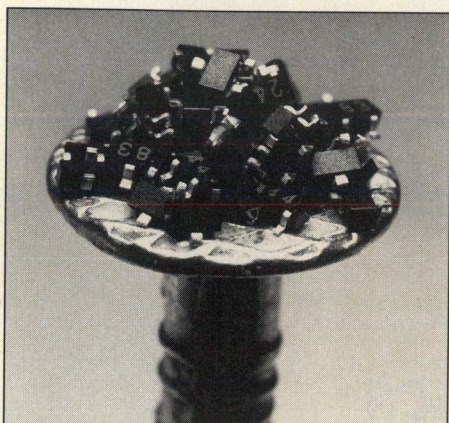
Figure 3. NE68519 packages on the head of a nail for size reference.
